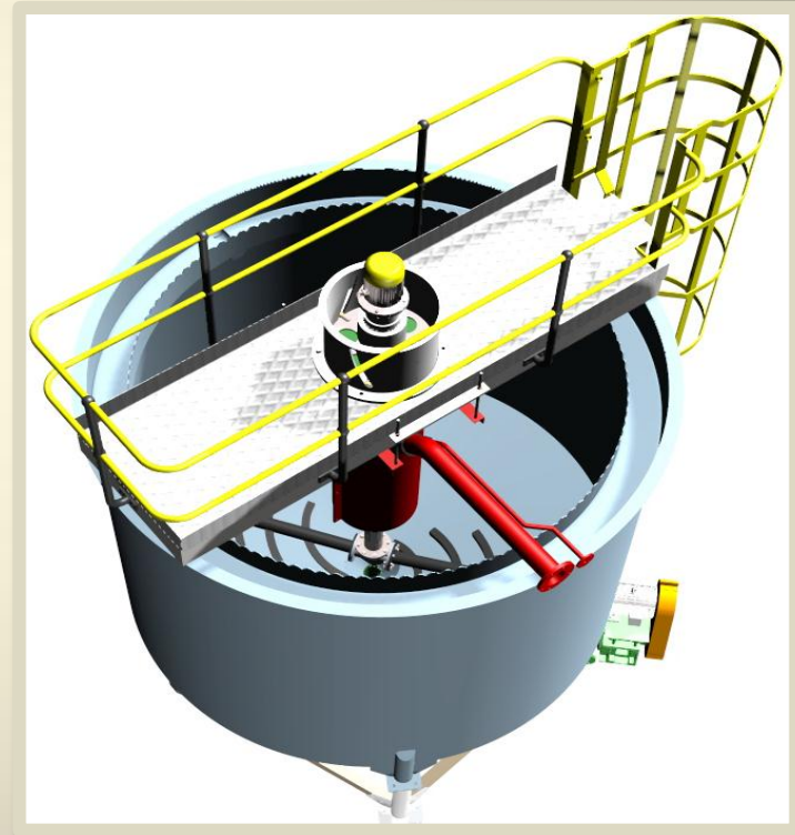
High rate thickener for process water recovery.
